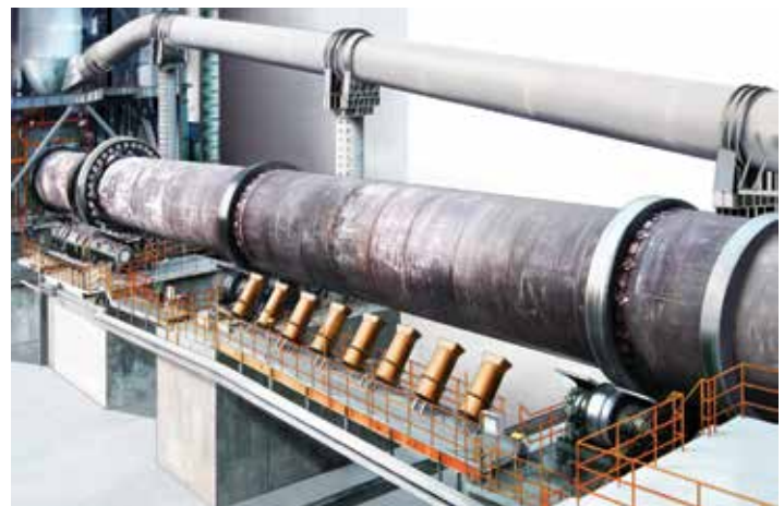
Cement Mill Kiln
