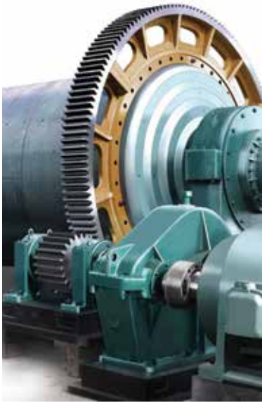
Cement Mill Mill-Gearing
